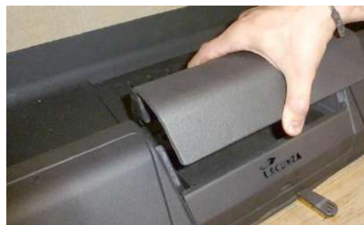
Figure No.23 - Removing the separator
