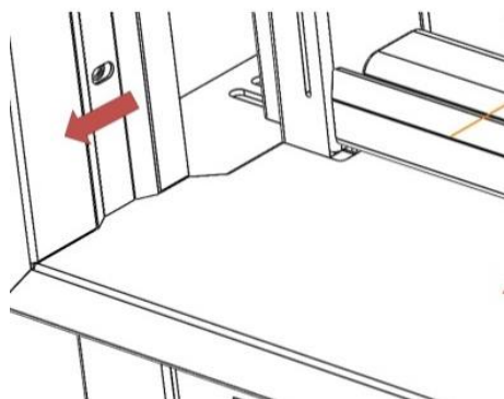
Figure No.7 - Removing the frame
